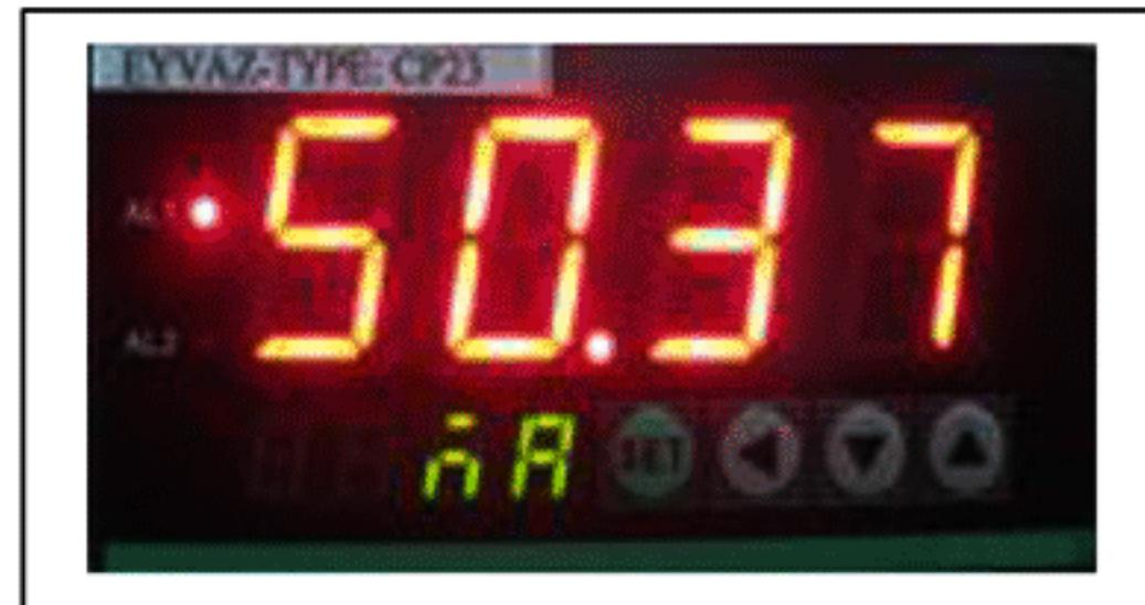
Display (0-100%). Moreover, this panel is programmable to define set point to send start/stop or alarm signal to steering circuit of pumps and alarm sets.
